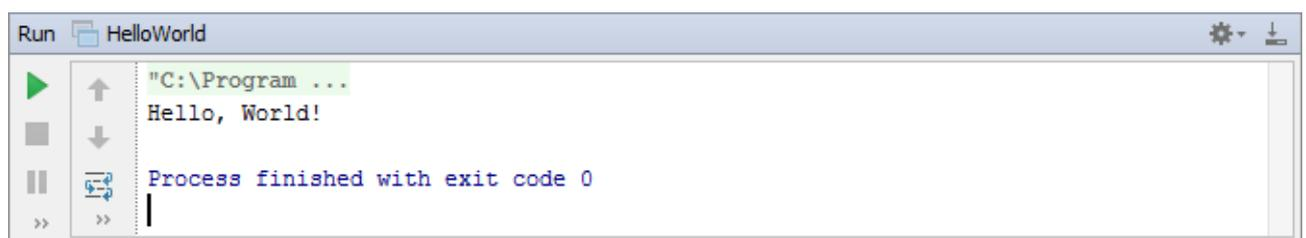
On the first line, a fragment of the command that IntelliJ IDEA used to run the class is shown. (Click the fragment to see the whole command line including all options and arguments.) The last line shows that the process has exited normally, and no infinite loops occurred. And, finally, you see the program output `Hello, World!` between these two lines.
